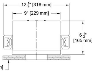
NOTE: This option is intended for use with precise and finished cutouts - usually millwork or wood ceilings. There is no plaster or finish flange.
